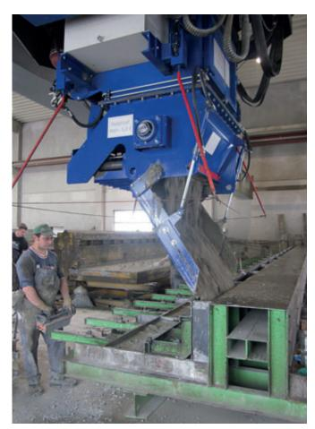
All mould heights can now be driven to flexibly and with the utmost accuracy by just one operator with the new concrete distributor.
